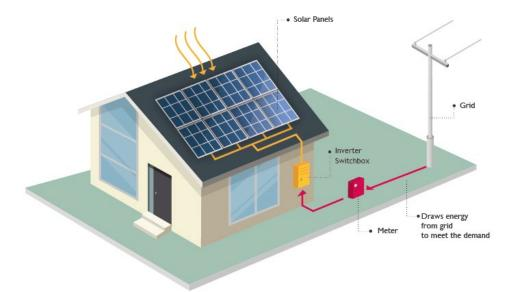
Figure 6 Behind-the-meter generator
