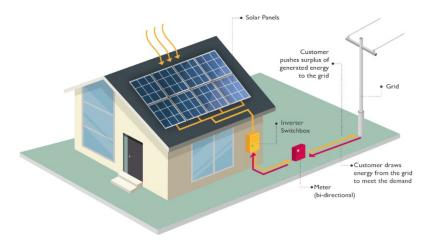
Figure 4 Household with a status of a Prosumer and solar PV installation
